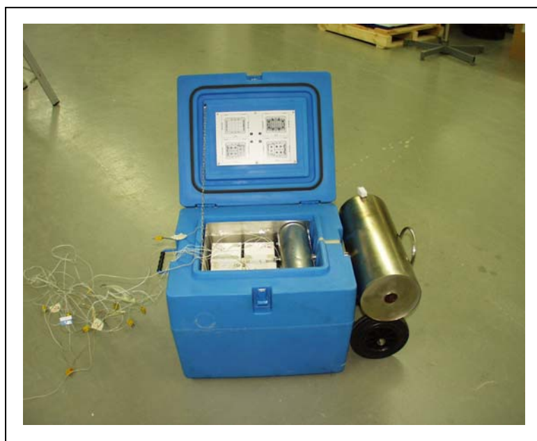
Figure 5. Prototype “Zeolite” intermittent cooler for passive containers
