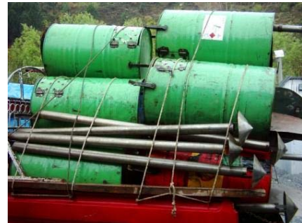
Several of the twenty drums incinerators on their way to remote health facilities in Balakot, to ensure proper disposal of medical waste
